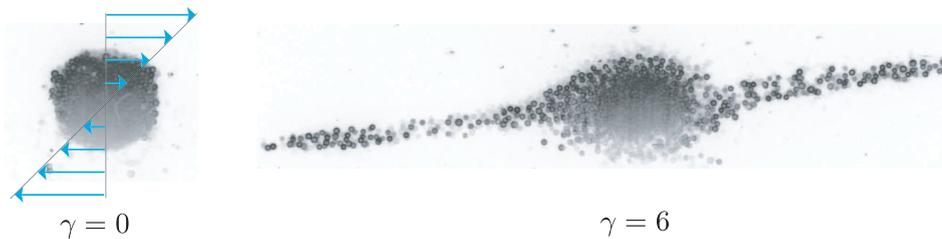
FIGURE V.3: *Perspectives – ‘Mixing’ an heterogeneity in a particulate suspension.* Blob with a large volume fraction of solid particles sheared in a liquid bath. Left: initial condition. Right: after 10 ‘back and forth’ shear cycles with a strain amplitude  $\gamma = 6$  (adapted from [130]).
